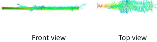
Figure 15. Direction of Min Principal stress on the heatsink section of drill path.
